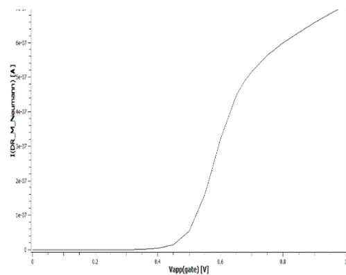
**Fig. 6 Transfer characteristics in linear scale for designed Heterojunction Device 3 FinFET structure with height 25nm and width 7nm**
