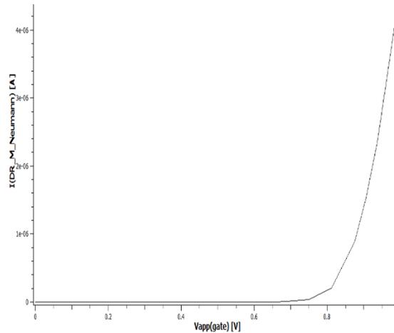
**Fig. 4 Transfer characteristics in linear scale for Heterojunction Device 1 FinFET structure at height 25nm and width 7nm.**
