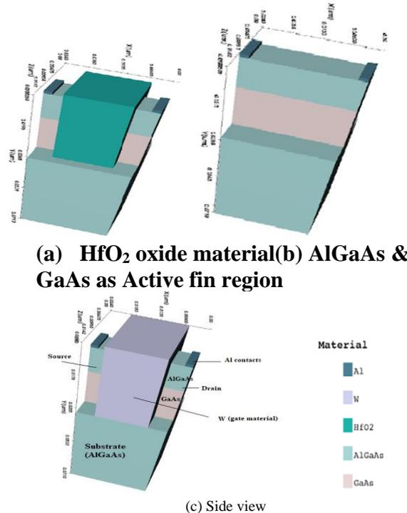
**Fig. 1: Hetero-junction Device 1 FinFET structure for height 25nm and Width 7nm**
