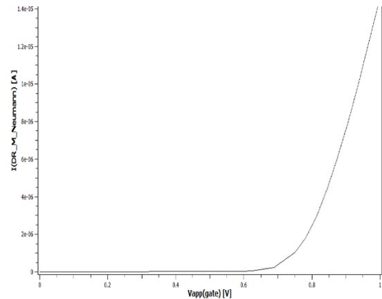
**Fig. 5 Transfer characteristics in linear scale for designed Heterojunction Device 2 FinFET structure with height 25nm and width 7nm.**
